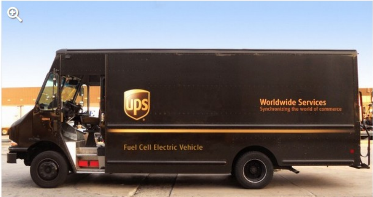
Prototype plug-in electric delivery van with fuel-cell range extender to be tested by UPS in 2017
